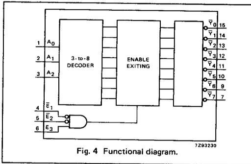
Fig. 4 Functional diagram.
