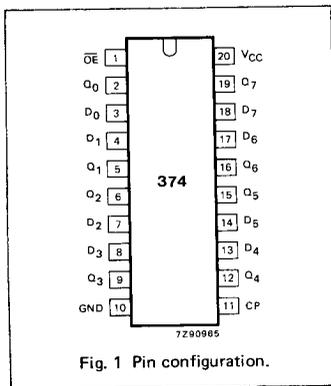
Fig. 1 Pin configuration.
