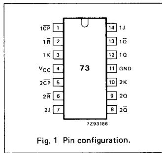
Fig. 1 Pin configuration.
