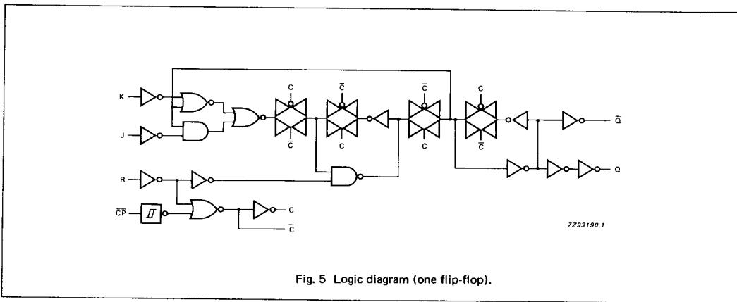
Fig. 5 Logic diagram (one flip-flop).
