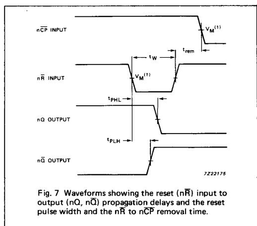
Fig. 7 Waveforms showing the reset ( $n\bar{R}$ ) input to output ( $nQ$ ,  $n\bar{Q}$ ) propagation delays and the reset pulse width and the  $n\bar{R}$  to  $n\bar{C}P$  removal time.
