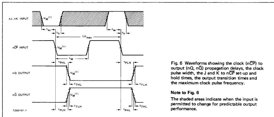
Fig. 6 Waveforms showing the clock ( $n\bar{C}P$ ) to output ( $nQ$ ,  $n\bar{Q}$ ) propagation delays, the clock pulse width, the J and K to  $n\bar{C}P$  set-up and hold times, the output transition times and the maximum clock pulse frequency.
