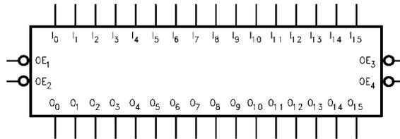
74LVT16244A • 74LVTH16244 Low Voltage 16-Bit Buffer/Line Driver with 3-STATE Outputs (Preliminary)
