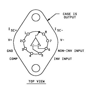
FIGURE 2. Terminal connections.
