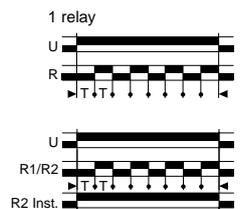
Function Di: the cycle begins with the output in the operating position. Pulse start.
