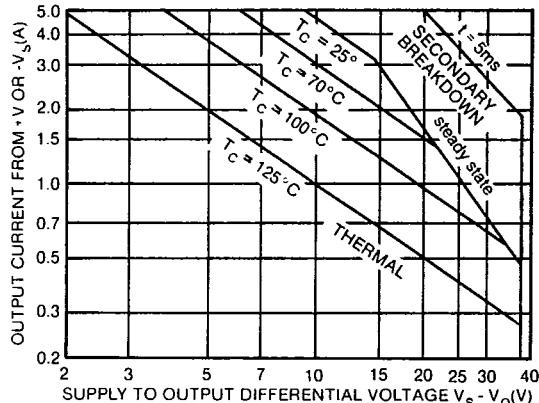
The SOA curves combine the effect of all limits for this Power Op Amp. For a given application, the direction and magnitude of the output current should be calculated or measured and checked against the SOA curves. This is simple for resistive loads but more complex for reactive and EMF generating loads. The following guidelines may save extensive analytical efforts:
