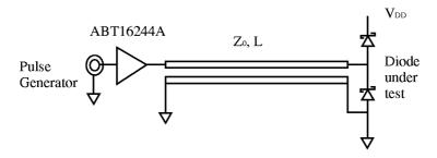
Test Circuit. Line length, pulse width and duty cycle are selected such as that only one reflection is involved in the measurement.
