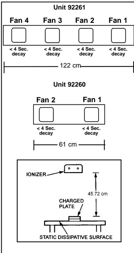
Figure 5. Balance under < 10 volts. When set under lab conditions, 5 volts is attainable.
