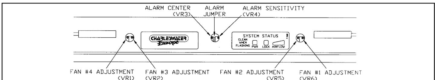
Figure 4. Calibrating C/E Ioniser
