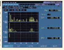
List Display of Harmonics The harmonic list display shows the amplitude, proportion, phase angle and distortion for each harmonic of voltage, current and power. Displaying only proportion, or two parameters simultaneously, such as amplitude and phase angle, is selectable.
