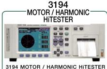
provides analysis of high-order harmonics up to the 3000th order. Additionally, with the optional 9603-01 EXTERNAL SIGNAL INPUT UNIT installed, the HiTESTER can directly measure torque and rotation speed, an essential feature for evaluating the performance of inverter motors. This makes it easy to construct measurement systems.
