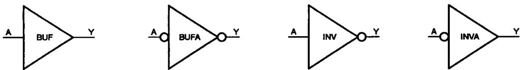
**I/O Buffers (I/O Module Count = 1)**
