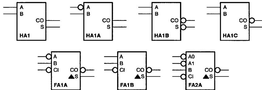
Macros FA1A, FA1B, and FA2A have two level delays from the inputs to the S outputs, as indicated by the ▲
