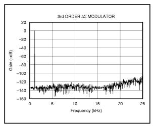
FIGURE 17. Quantization Noise Spectrum.
