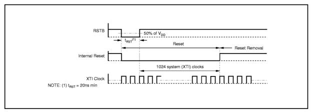
FIGURE 14. RSTB-Pin Reset Timing.
