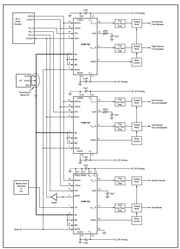
FIGURE 18. Connection Diagram for a 6-Channel AC-3 Application.
