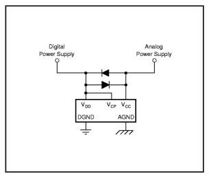
FIGURE 15. Latch-up Prevention Circuit.
