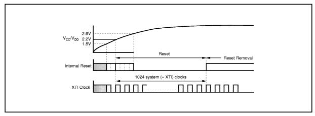
FIGURE 13. Internal Power-On Reset Timing.
