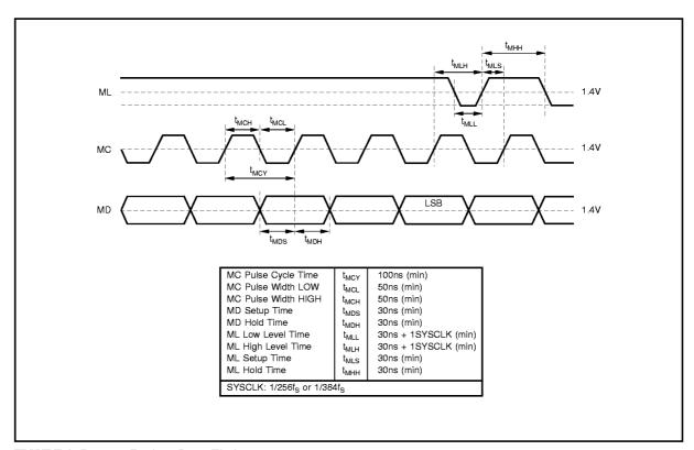
FIGURE 9. Program Register Input Timing.
