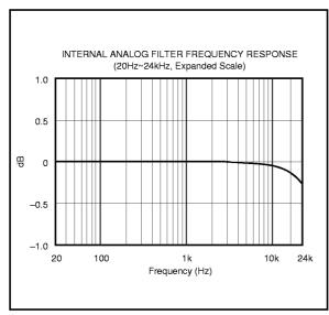
FIGURE 10. Low Pass Filter Frequency Response.
