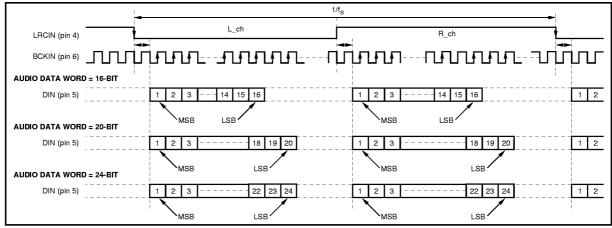
FIGURE 6. "I2S" Data Input Timing.
