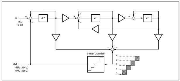
FIGURE 16. 5-Level  $\Delta\Sigma$  Modulator Block Diagram.
