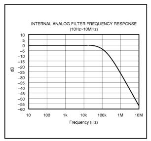
FIGURE 11. Low Pass Filter Wideband Frequency Response.
