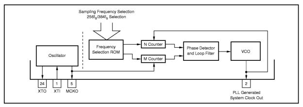
FIGURE 2. PLL Block Diagram.
