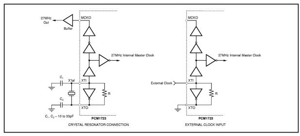
FIGURE 4. System Clock Connection.
