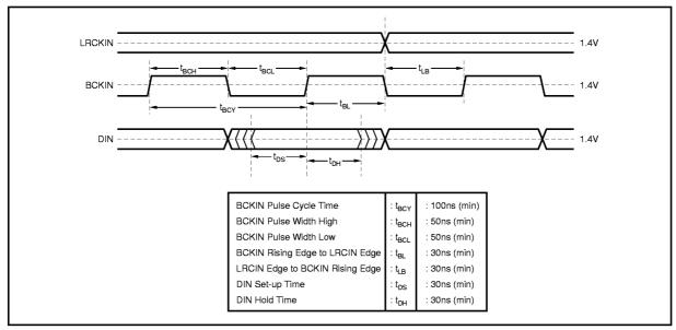
FIGURE 7. Audio Data Input Timing.
