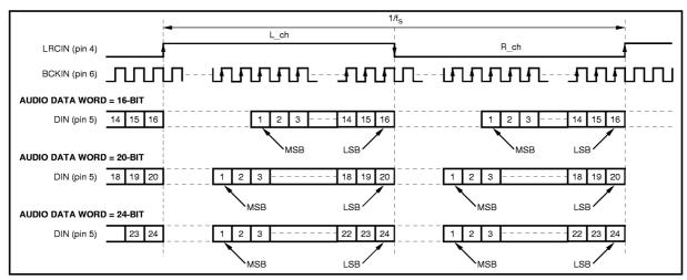
FIGURE 5. "Normal" Data Input Timing.
