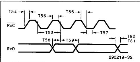
Figure 59. Receive Data Waveforms (NRZ)
