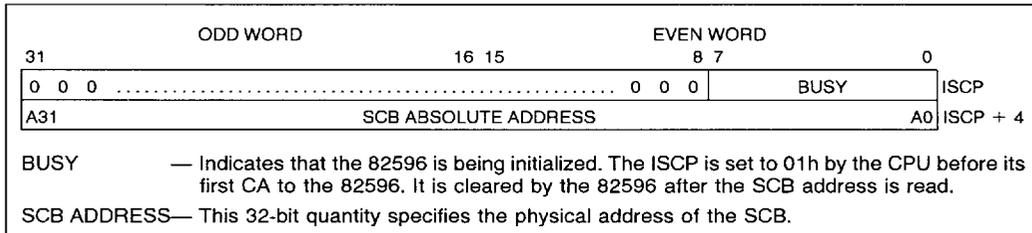
**Figure 17. The Intermediate System Configuration Pointer—Linear Mode.**
