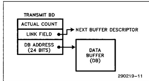
**Figure 11. Data Buffer Descriptor and Data Buffer Structure**
