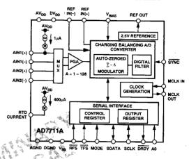
CMOS construction ensures low power dissipation and a software programmable power down mode reduces the standby power consumption to only 7 mW typical. The part is available in a 24-pin, 0.3 inch-wide, plastic and hermetic dual-in-line package (DIP) as well as a 24-lead small outline (SOIC) package.
