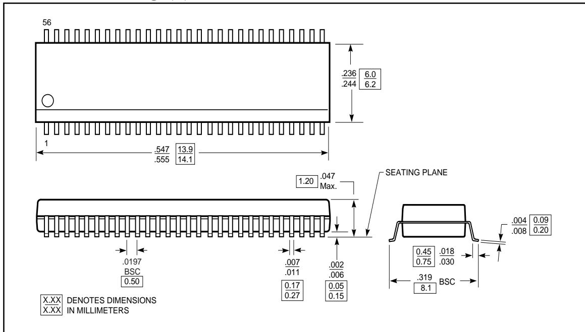
**56-Pin SSOP Package (V)**
