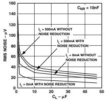
Figure 18. RMS Noise vs.  $C_L$  (10 Hz–100 kHz)
