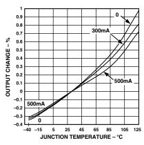
Figure 6. Output Voltage Variation % vs. Junction Temperature
