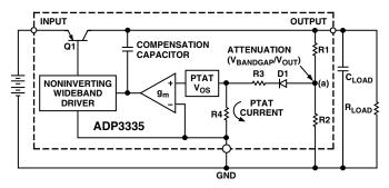
Figure 20. Functional Block Diagram
