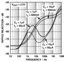
Figure 17. Power Supply Ripple Rejection
