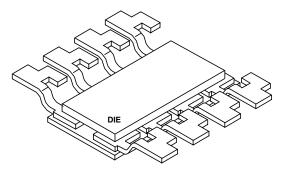
Figure 22. Thermally Enhanced Paddle-Under-Lead Package
