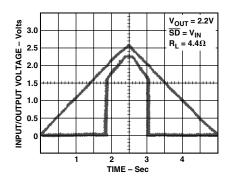
Figure 9. Power-Up/Power-Down
