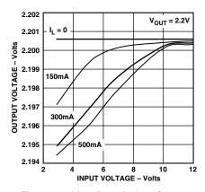
Figure 2. Line Regulation Output Voltage vs. Supply Voltage
