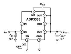
Figure 21. Typical Application Circuit
