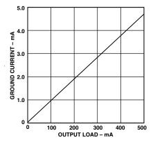
Figure 5. Ground Current vs. Load Current
