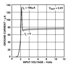
Figure 4. Ground Current vs. Supply Voltage
