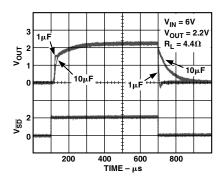
Figure 14. Load Transient Response
