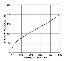
Figure 8. Dropout Voltage vs. Output Current
