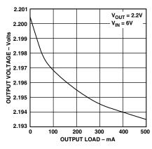
Figure 3. Output Voltage vs. Load Current
