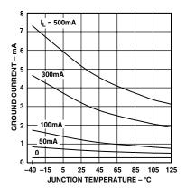
Figure 7. Ground Current vs. Junction Temperature
