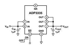
Figure 1. Typical Application Circuit
