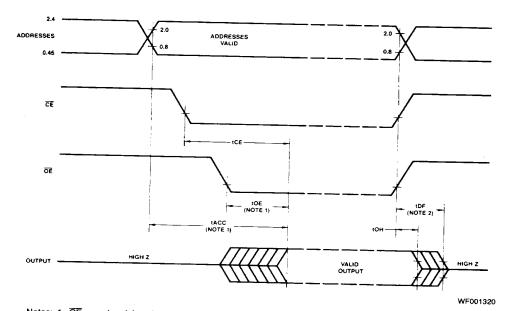
Notes: 1.  $\overline{\text{OE}}$  may be delayed up to  $t_{\text{ACC}}$  -  $t_{\text{OE}}$  after the falling edge of  $\overline{\text{OE}}$  without impact on  $t_{\text{ACC}}$ . 2.  $t_{\text{DF}}$  is specified from  $\overline{\text{OE}}$  or  $\overline{\text{CE}}$ , whichever occurs first.
