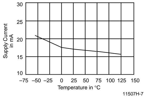
**Figure 2. Typical Supply Current vs. Temperature**
