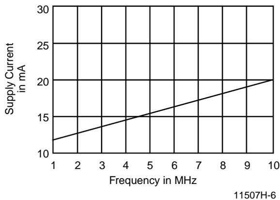
**Figure 1. Typical Supply Current vs. Frequency**
