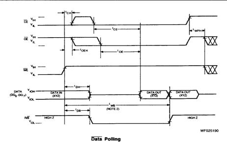
Notes: 1. This is shown for single byte write. In page write,  $R/\overline{B}$  goes LOW on first LOW-to-HIGH transition of  $\overline{WE}$ .
