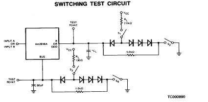
$^{*}C_{L}$  = 15pF for tpLH, tpHL, tzL, tzH  $C_{L}$  = 5pF for tHz, tLZ
