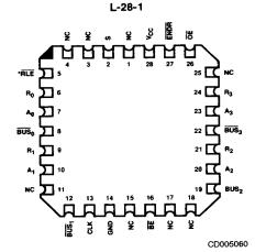
Note: Pin 1 is marked for orientation \*ENREC for Am2928
