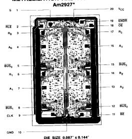
NOTE: The Am2928 is similar to the Am2927, but with a D-type edge-triggered register in the receiver and a receiver enable, ENREC, which functions as a common clock enable.
