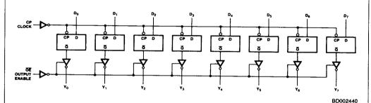
Inputs D<sub>0</sub> through D<sub>7</sub> are inverted on the Am2955.
