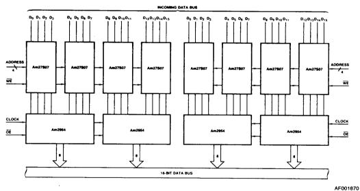
Dual 16-word by 16-bit non-inverting high-speed data buffer.
