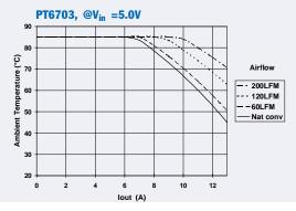
**Note A:** Characteristic data has been developed from actual products tested at 25°C. This data is considered typical data for the Converter. **Note B:** SOA curves represent the conditions at which internal components are at or below the manufacturer's maximum operating temperatures
