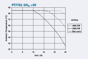
Note A: Characteristic data in the above graphs has been developed from actual products tested at 25°C. This data is considered typcial for the ISR. Note B: SOA curves represent conditions at which internal components are at or below manufacturer's maximum operating temperatures.
