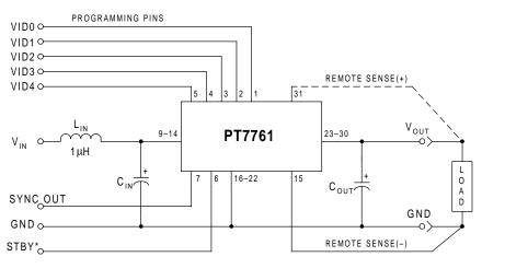
$C_{in}$  = Required 1500µF electrolytic  $C_{out}$  = Required 330µF electrolytic
