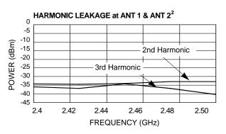
2. Measured with an RF input power of -3 dBm at PA IN. Output measured at ANT 1 and ANT 2 with PA OUT and ANT COMMON terminated in  $50\Omega.$
