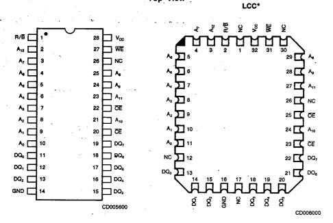
Note: Pin 1 is marked for orientation.
