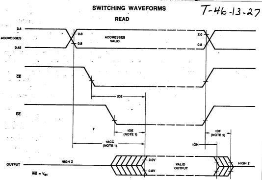
Notes: 1.  $\overline{\text{OE}}$  may be delayed up to tACC-tOE after the falling edge of  $\overline{\text{CE}}$  without impact on tACC.
