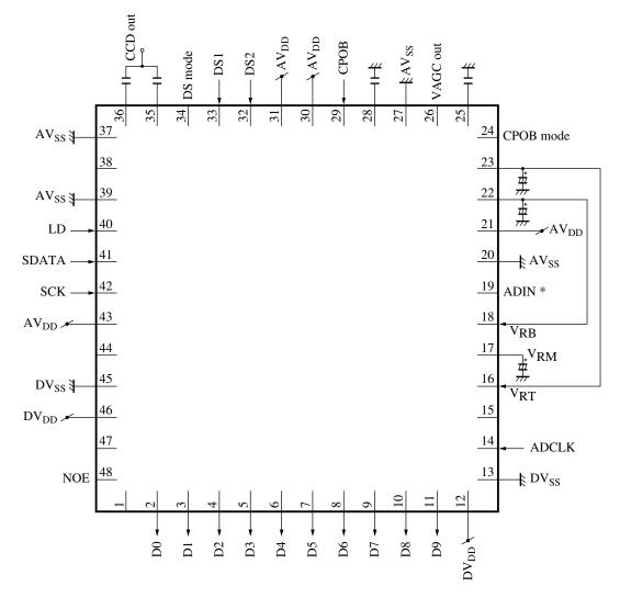
Note \*: When the AD amplifier is used, signals should be input to pin 19 through a capacitor. (Assumed chrominance signal may be input.)
