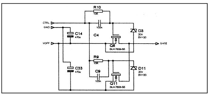
Fig. 3 Simplified version of gdu turn-off section - in reality 10x 470µF capacitors used
