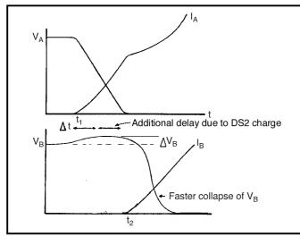
Fig. 2 Turn-on waveforms
