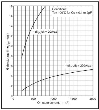
Fig. 7 Gate storgae time vs on-state current
