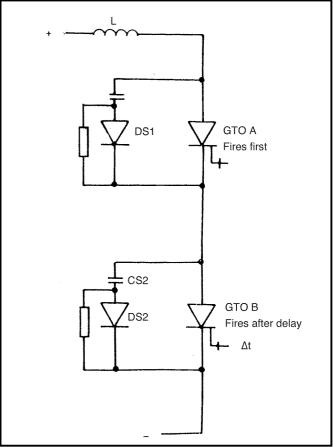
Fig. 1 GTOs in series with snubber networks
