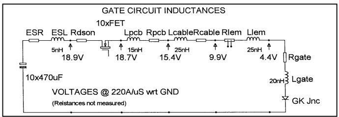
Fig. 4 Loop inductance and dynamic resistance
