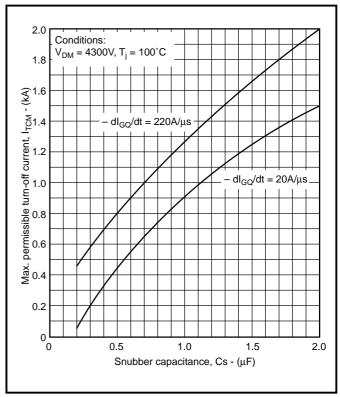
Fig. 6 Max. permissible turn-off current vs snubber capacitance
