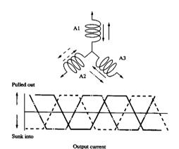
The AN8293SA employs highly effective three-phase full-wave system, by which current is pulled out or sunk from/into each phase, A1, A2 and A3.
