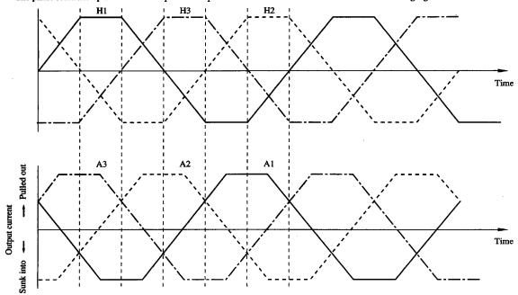
When EC>ECR, the pulling-out and sinking-into of the output current is just reversed from those shown in the above figure, and the motor rotation direction is reversed.
