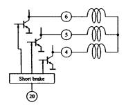
As shown in the left figure, when high signal is applied to the brake terminal, the lower side transistors are turned on to set the motor coil to the short condition and the brake operation is executed.
