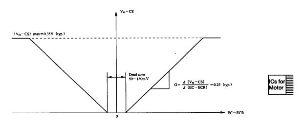
The G shown in the above figure and  $(V_M - CS)$  max, are almost stable, independent of current detection resistance (resistance between  $V_M$  and CS terminals),  $R_{CS}$ . For example, if  $R_{CS} = 1 \Omega$ ,
