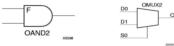
Figure 21: AND & MUX Symbols in XC4000X IOB
