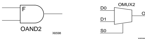
Figure 7: AND & MUX Symbols in Spartan-XL IOB
