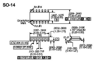
14-Lead SOP outline dimensions Narrow body .150 (All dimensions per JECEC No. MS-012-AB, issue C) Omensions in ( ) are in mm.
