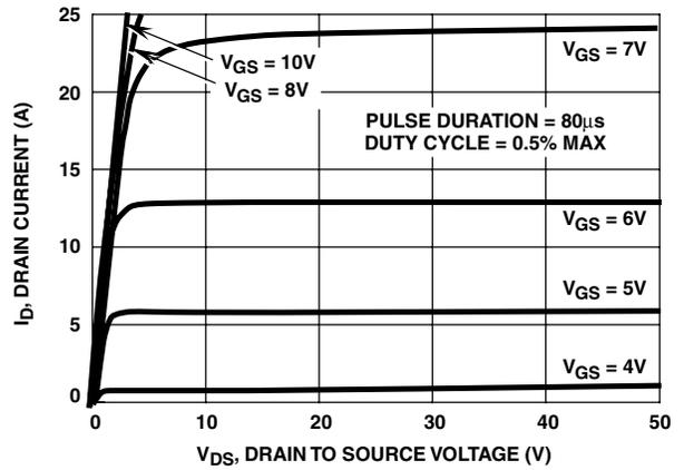
FIGURE 5. OUTPUT CHARACTERISTICS
