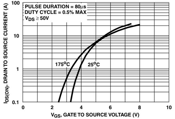
FIGURE 7. TRANSFER CHARACTERISTICS
