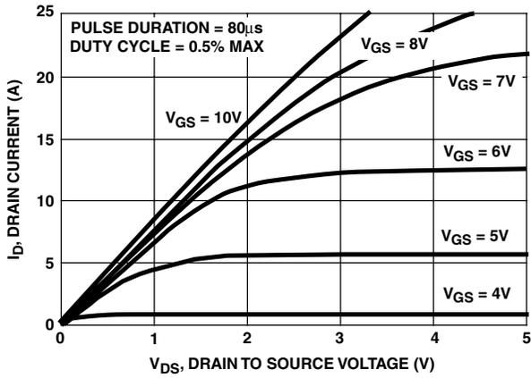
FIGURE 6. SATURATION CHARACTERISTICS
