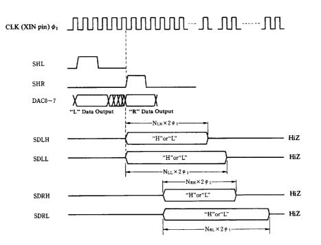
However, NLH, NLL, NRH, and NRL are the number of bits of the absolute value of the difference of the previous sound data. If it is larger than the previous data, the output value is "H", and if it is smaller, the output value is "L"
