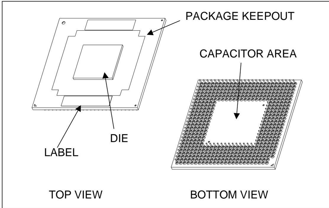
Figure 23. Socketable Micro-FCPGA Package - Top and Side View
