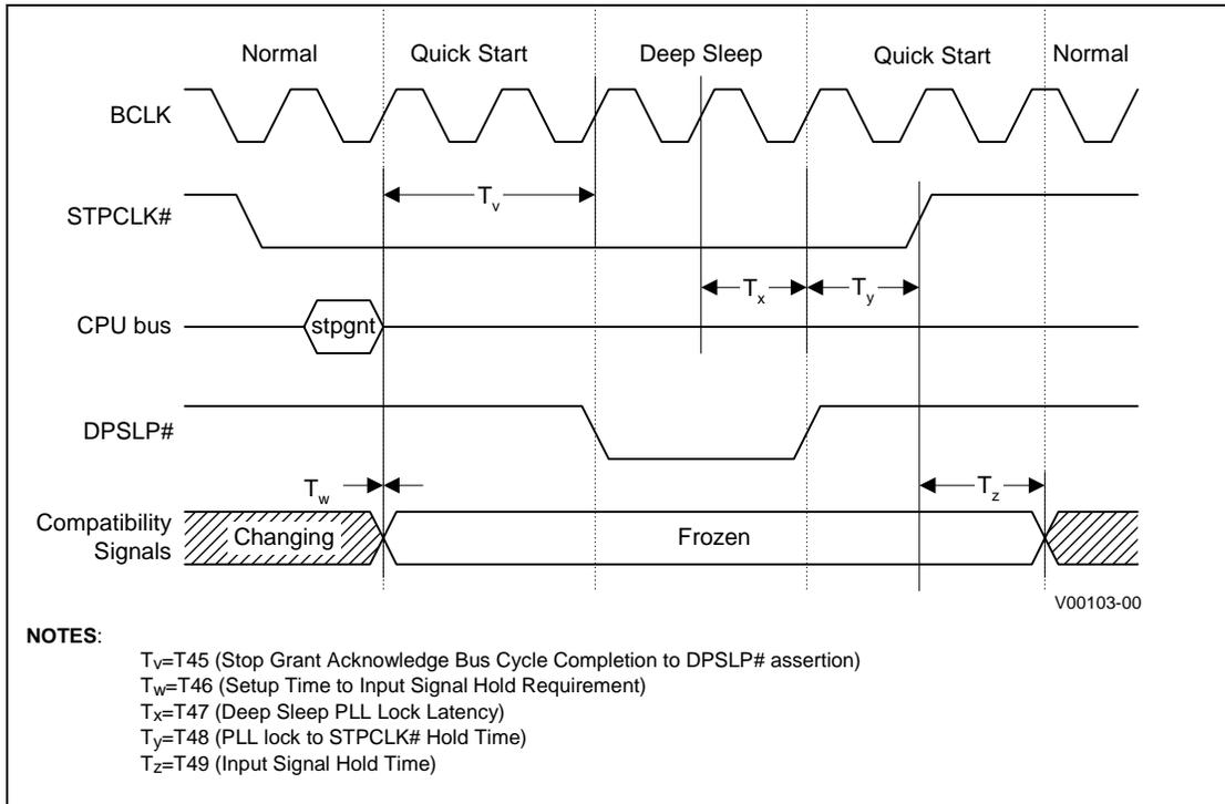
**Figure 19. Enhanced Intel SpeedStep Technology/Deep Sleep Timing**
