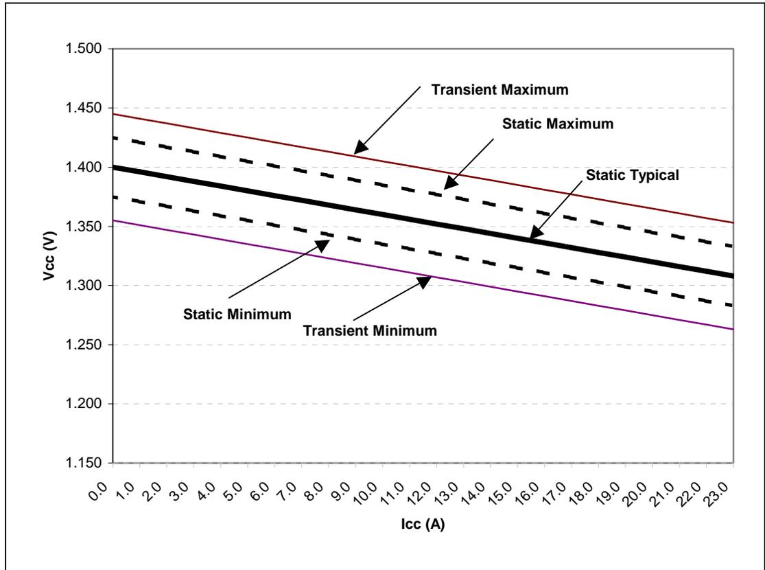
**Table 11. V<sub>CC</sub> Tolerances for the Mobile Intel Pentium III Processor-M in the Deep Sleep State: VID = 1.40V (Performance Mode) and 1.15V (Battery Optimized Mode)**
