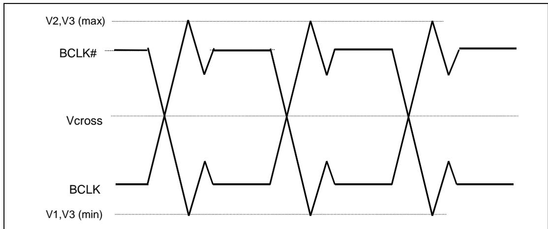
Figure 8. BCLK/BCLK# Waveform (Differential Mode)
