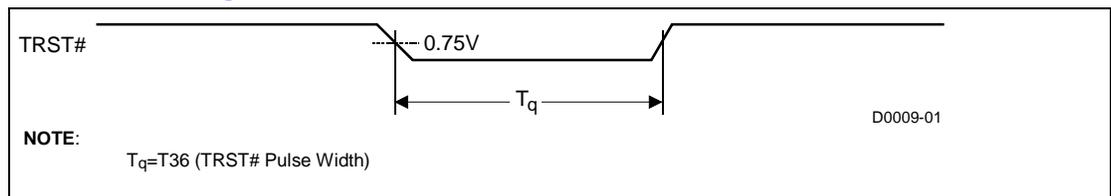
Figure 17. Quick Start/Deep Sleep Timing (BCLK Stopping Method)
