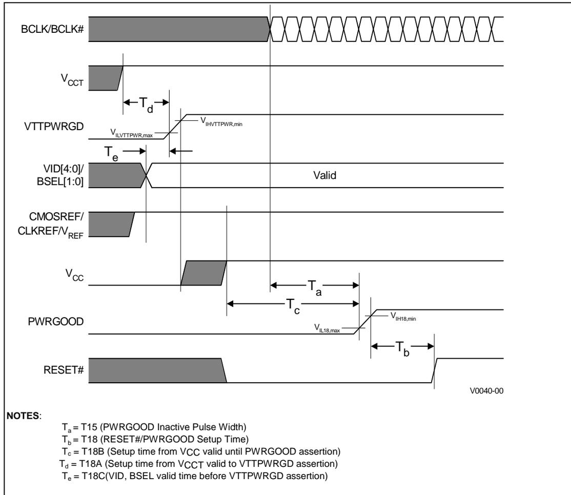
Figure 13. Power Down Sequencing and Timings (VCC Leading)
