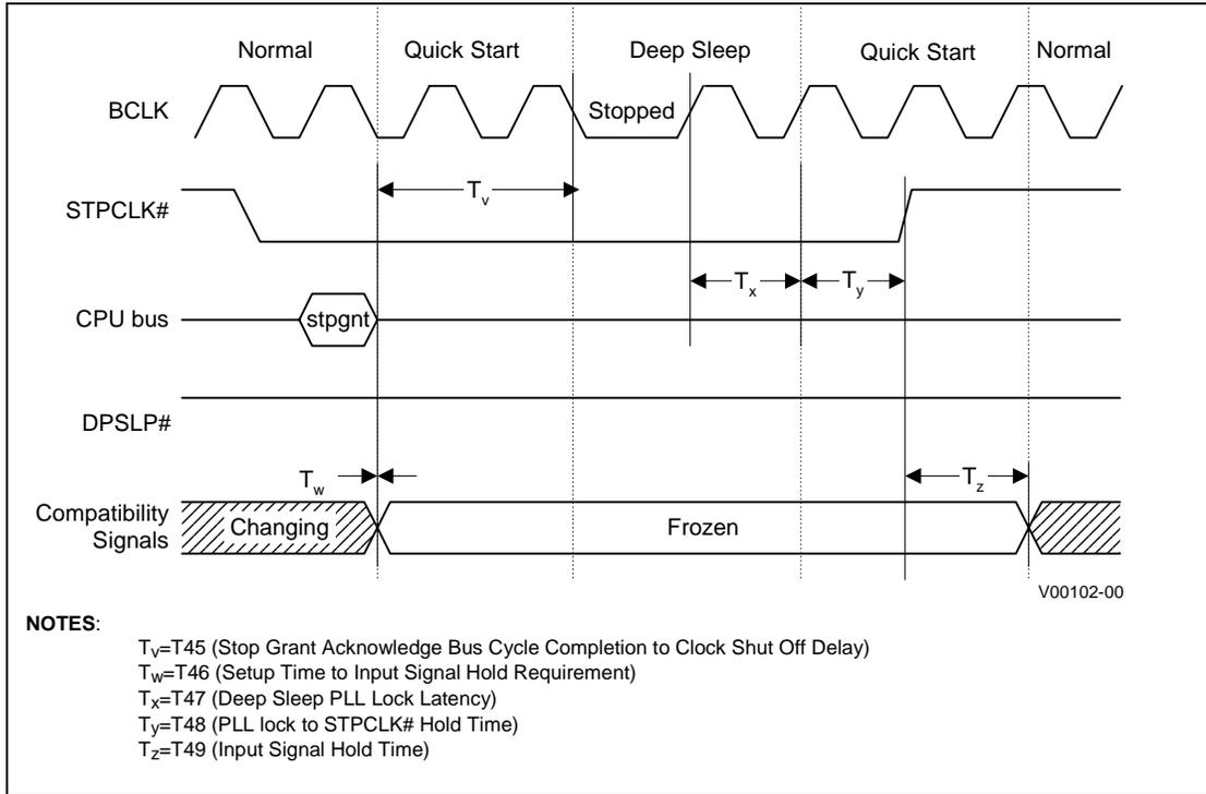
Figure 18. Quick Start/Deep Sleep Timing (DPSLP# Assertion Method)
