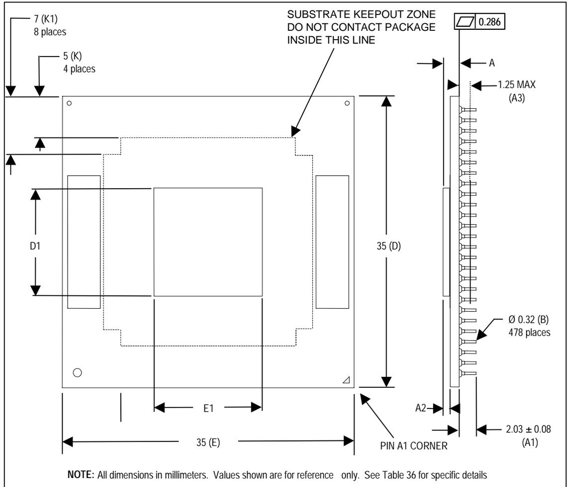
Figure 24. Socketable Micro-FCPGA Package - Bottom View
