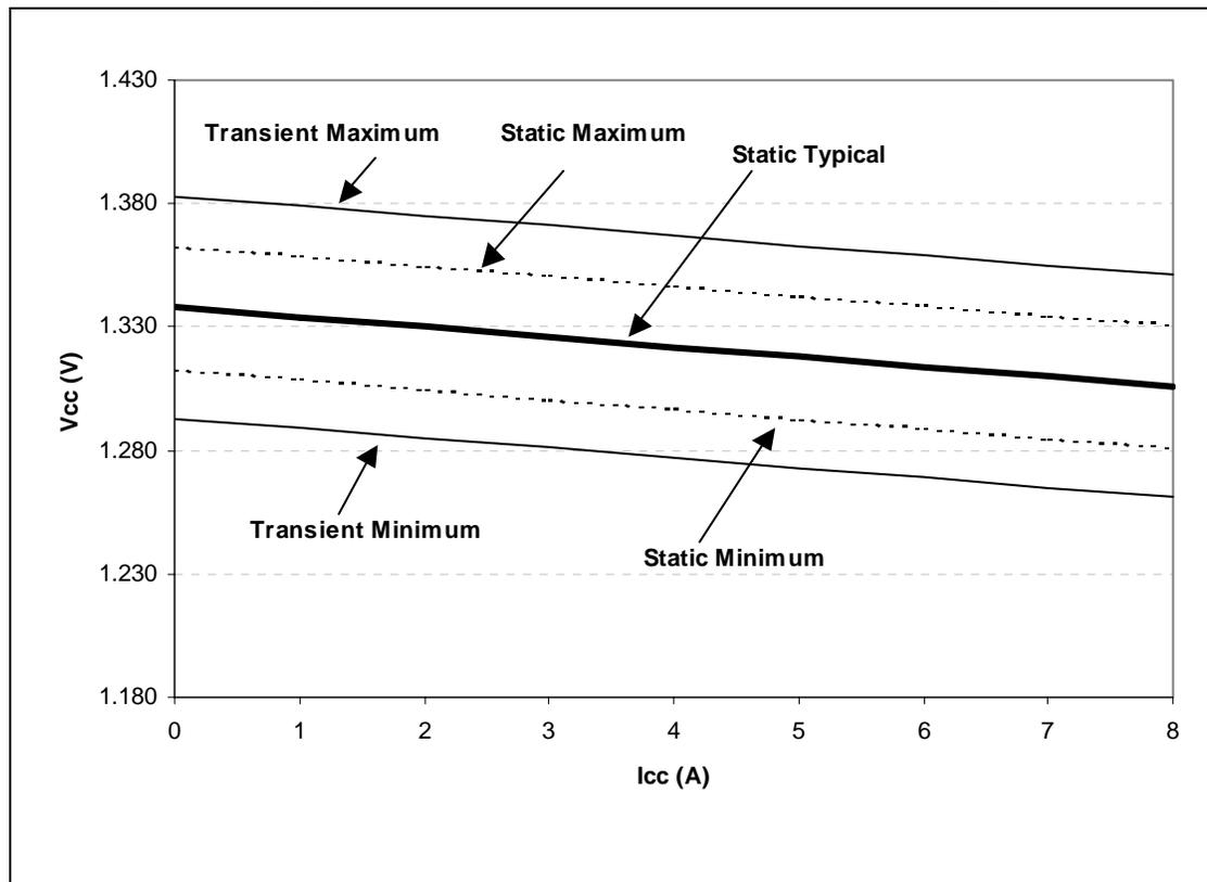
**Table 12.  $V_{CC}$  Tolerances for the Low Voltage Mobile Intel Pentium III Processor-M: VID = 1.15V (Performance Mode) and 1.05V (Battery Optimized Mode)**
