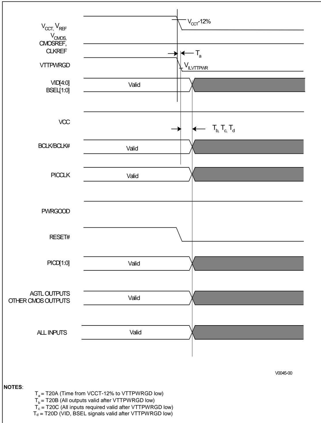
**Figure 15. Test Timings (Boundary Scan)**
