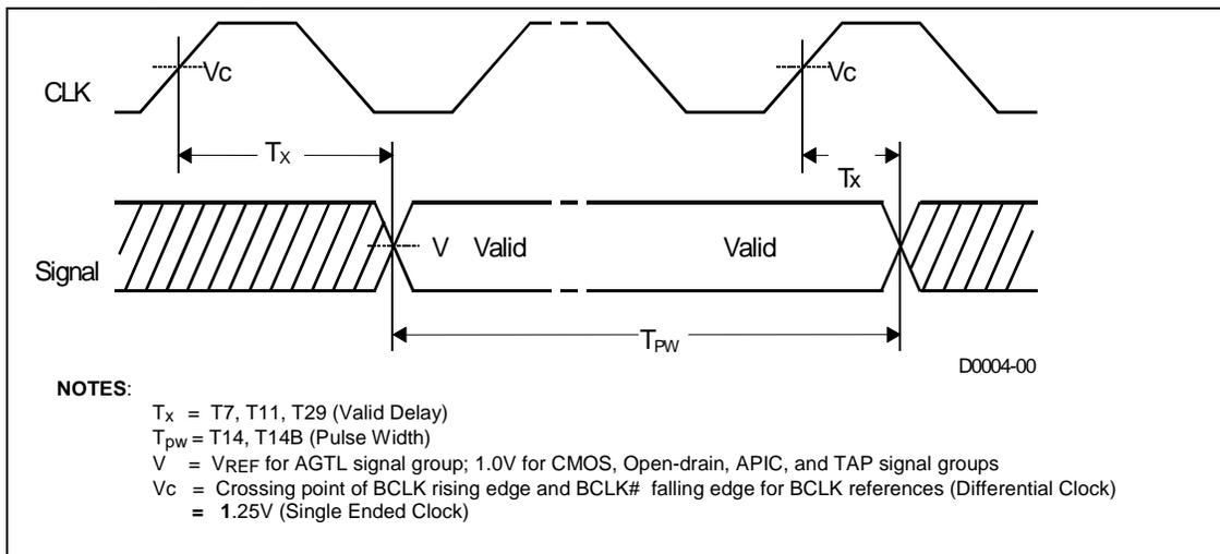
Figure 10. Setup and Hold Timings
