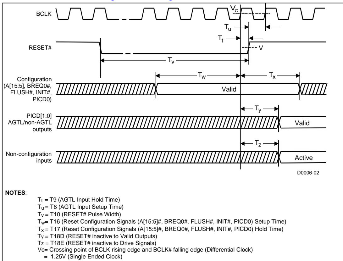
Figure 12. Power-on Sequence and Reset Timings
