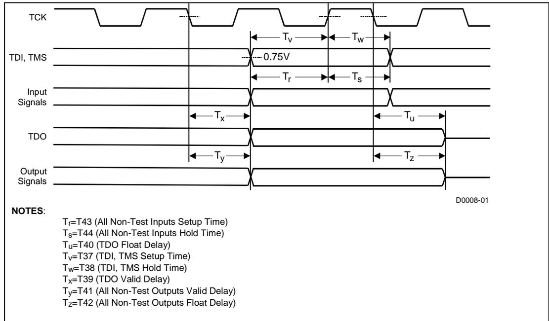
**Figure 16. Test Reset Timings**
