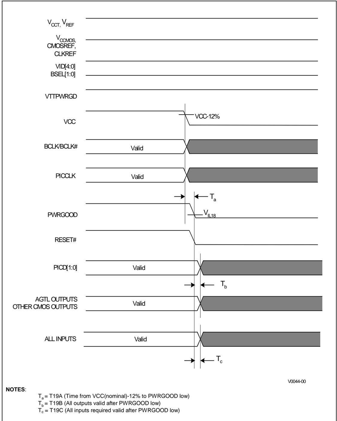
Figure 14. Power Down Sequencing and Timings ( $V_{CCT}$  Leading)
