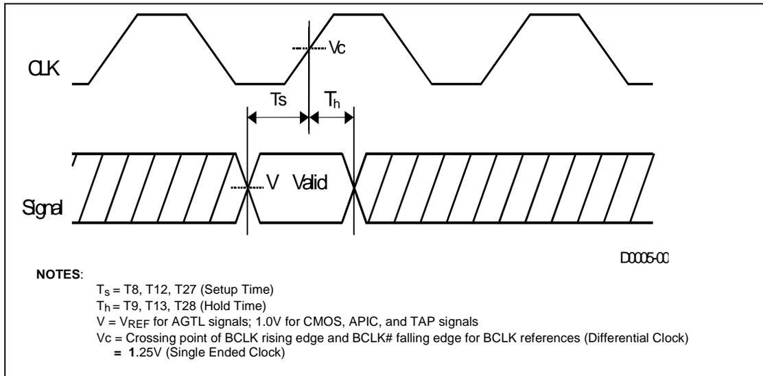
Figure 11. Cold/Warm Reset and Configuration Timings
