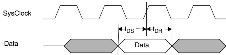
**Figure 13 Output Timing**
