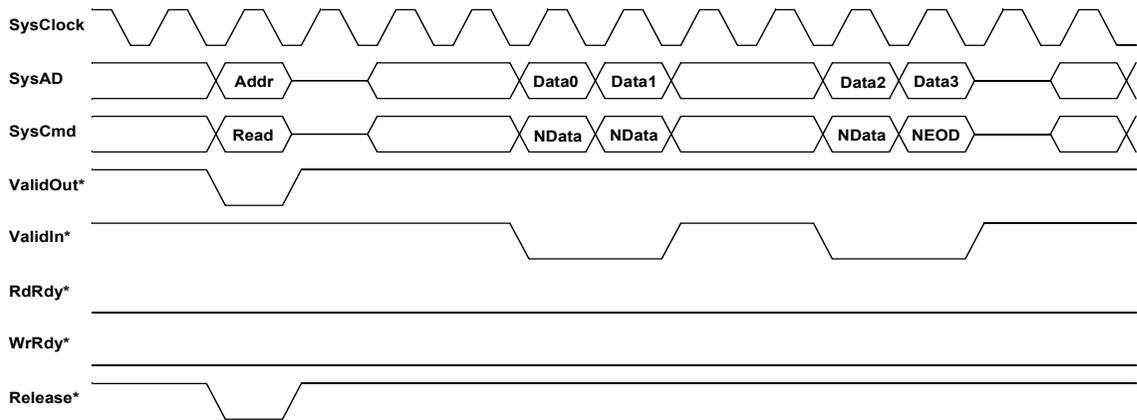
In Figure 8 the read latency is 4 cycles (**ValidOut\*** to **ValidIn\***), and the response data pattern is DDxxDD. Figure 9 shows a processor block write where the processor was programmed with write-back data rate boot code 2, or DDxxDDxx.
