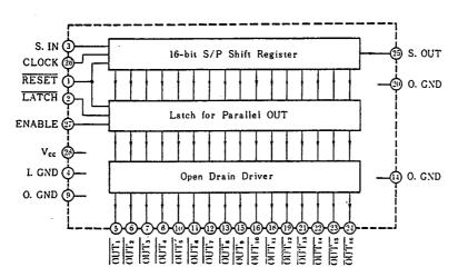
NOTE: The GND for open drain transistors is provided separately from that (I. GND) for the logic circuit because it should allow large current to flow.
