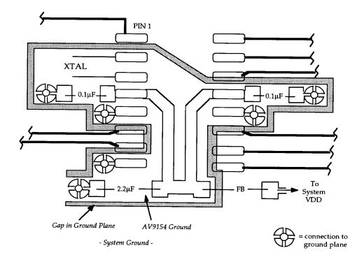
This is the recommended layout for the AV9154 to maximize clock performance. Shown are the power and ground connections, the ground plane, and the input/output traces.
