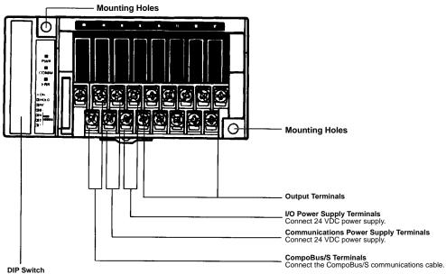
Used for node number setting and holding or clearing outputs for communications error.
