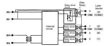
Note: The G3DZ-2R6PL Power MOSFET Relay is inserted into this portion of the SRT□-R0F08 and SRT□-R0F16.
