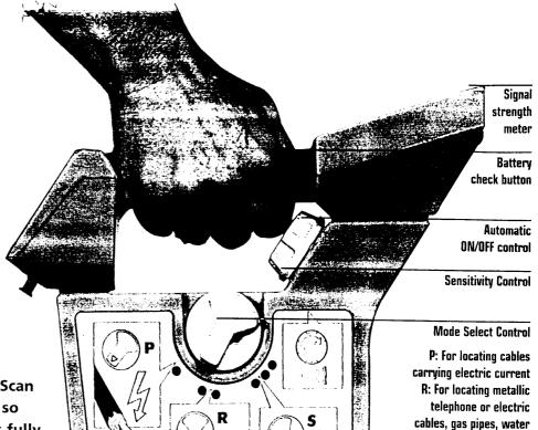
In Scansmitter mode the U-Scan has a dual frequency capability so that, should the need arise, it is fully compatible with other leading makes of cable detection equipment. Step-by-Step diagrammatic operating instructions are printed on the side of the machine for instant on-site reference.
