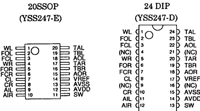
Two types of compact packages, 20SSOP(YSS247-E) and 24DIP(YSS247-D) are available.
