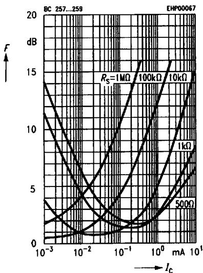
**Noise figure  $F = f(I_C)$**  $V_{CE} = 5 \text{ V}, f = 1 \text{ Hz}$
