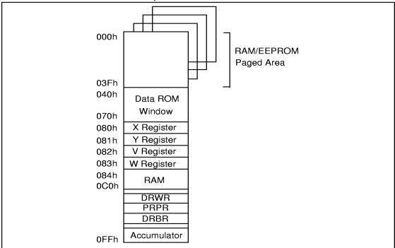
You must define the characteristics of each byte that you want to use in the data space using the .DEF directive (see "DEF - Define Data Space Location Characteristics" on page 62). This includes the standard registers listed above. .DEF enables you to associate a label with an address and define the following characteristics:
