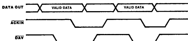
Figure 22. Interlocked Handshake Timing (Output) Port 2 Side Only
