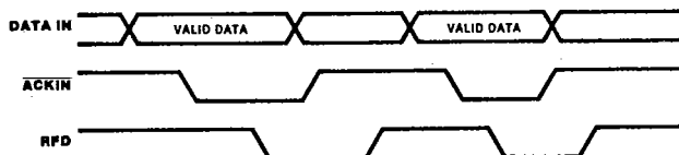
Figure 21. Interlocked Handshake Timing (Input) Port 2 Side Only
