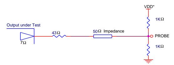
NOTE: All buffer outputs are tied to a common 3.3 Volt VDD (VDD\*) for testing purposes
