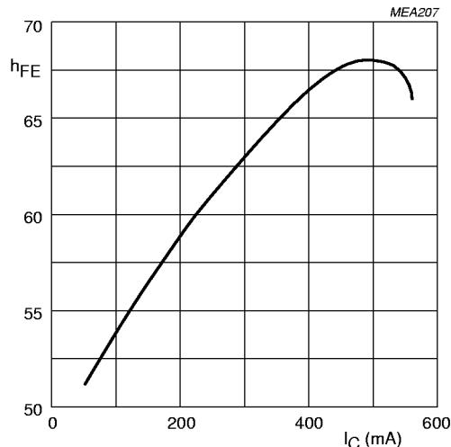
$V_{CE} = 5$  V;  $T_{amb} = 25$  °C.
