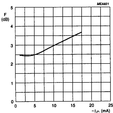
$V_{CE} = -10$  V;  $Z_S = \text{opt.}$ ;  $f = 500$  MHz;  $T_{amb} = 25$  °C.
