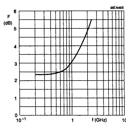
$I_C = -2$  mA;  $V_{CE} = -10$  V;  $Z_S = \text{opt.}$ ;  $T_{amb} = 25$  °C.
