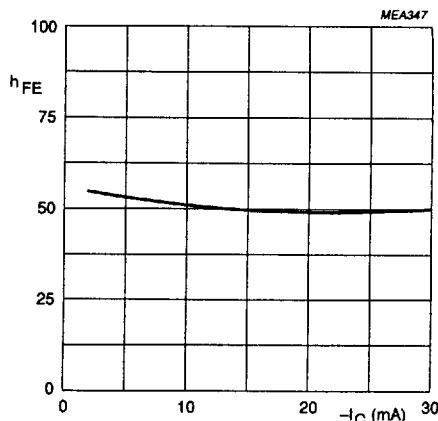
$V_{CE} = -10 \text{ V}; T_j = 25^\circ\text{C}$ .
