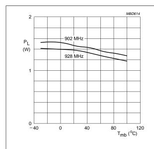
$Z_S$  =  $Z_L$  = 50  $\Omega;~P_D$  = 2 mW;  $V_S$  = 6 V;  $V_C$  = 3.5 V.
