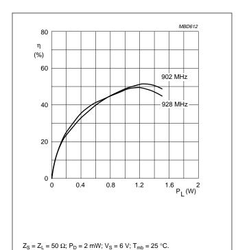
Fig.24 Efficiency as a function of load power; BGY115D, typical values.
