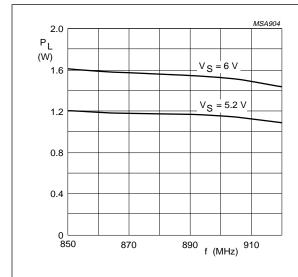
$Z_S$  =  $Z_L$  = 50  $\Omega;$   $P_D$  = 2 mW;  $V_C$  = 3.5 V;  $T_{mb}$  = 25  $^{\circ}C.$
