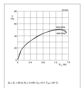
Fig.3 Efficiency as a function of load power; BGY115A, typical values.
