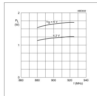
Fig.18 Load power as a function of frequency; BGY115C/P, typical values.
