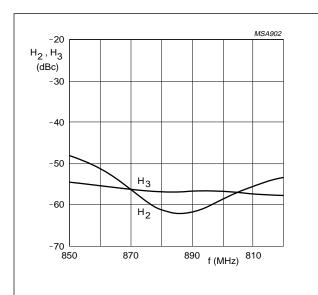
$Z_S$  =  $Z_L$  = 50  $\Omega;$   $P_D$  = 2 mW;  $P_L$  = 1.2 W;  $V_S$  = 6 V;  $T_{mb}$  = 25  $^{\circ}C.$
