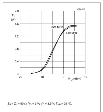
Fig.7 Load power as a function of drive power; BGY115A, typical values.
