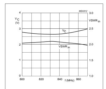
$Z_S$  =  $Z_L$  = 50  $\Omega$ ;  $P_D$  = 2 mW;  $P_L$  = 1.2 W;  $V_S$  = 6 V;  $T_{mb}$  = 25 °C.
