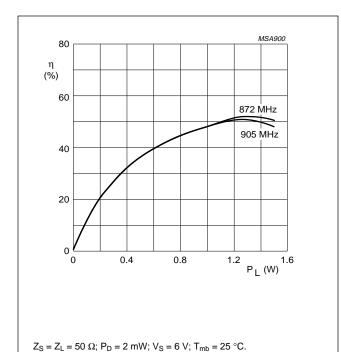
Fig.10 Efficiency as a function of load power; BGY115B, typical values.
