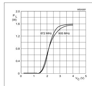
$Z_S$  =  $Z_L$  = 50  $\Omega$ ;  $P_D$  = 2 mW;  $V_S$  = 6 V;  $T_{mb}$  = 25  $^{\circ}C$ .
