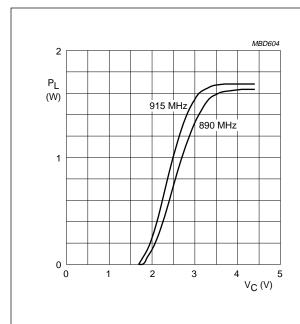
$Z_S = Z_L = 50~\Omega; \, P_D = 2~\text{mW}; \, V_S = 6~\text{V}; \, T_{mb} = 25~^{\circ}\text{C}.$
