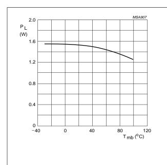
$Z_S$  =  $Z_L$  = 50  $\Omega;$   $P_D$  = 2 mW;  $V_S$  = 6 V;  $V_C$  = 3.5 V; f = 890 MHz.
