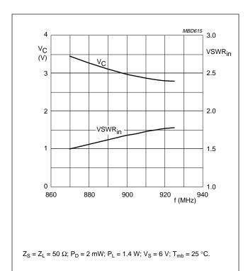
Fig.20 Control voltage and VSWR input as functions of frequency; BGY115C/P, typical values.
