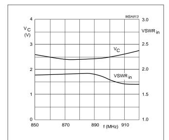
$Z_S$  =  $Z_L$  = 50  $\Omega;$   $P_D$  = 2 mW;  $P_L$  = 1.2 W;  $V_S$  = 6 V;  $T_{mb}$  = 25  $^{\circ}C.$
