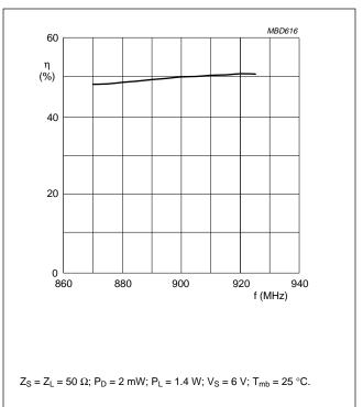
Fig.21 Efficiency as a function of frequency; BGY115C/P, typical values.
