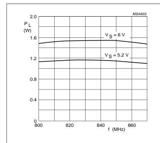
$Z_S$  =  $Z_L$  = 50  $\Omega;$   $P_D$  = 2 mW;  $V_C$  = 3.5 V;  $T_{mb}$  = 25  $^{\circ}C.$
