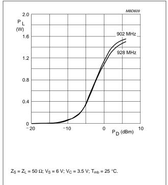
Fig.28 Load power as a function of drive power; BGY115D, typical values.
