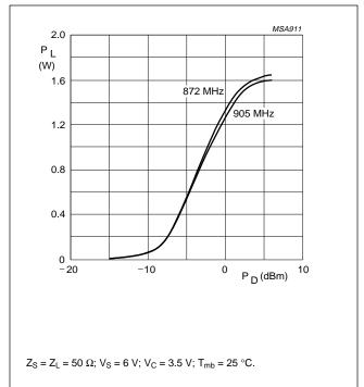
Fig.14 Load power as a function of drive power; BGY115B, typical values.
