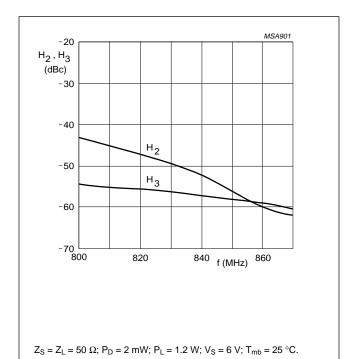
Fig.8 Harmonics as functions of frequency; BGY115A, typical values.
