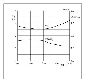
$Z_S$  =  $Z_L$  = 50  $\Omega;$   $P_D$  = 2 mW;  $P_L$  = 1.2 W;  $V_S$  = 6 V;  $T_{mb}$  = 25  $^{\circ}C.$
