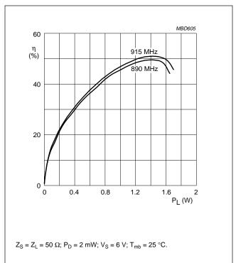
Fig.17 Efficiency as a function of load power; BGY115C/P, typical values.
