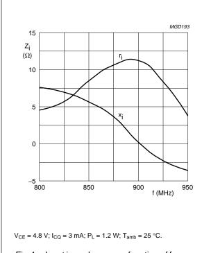
Input impedance as a function of frequency (series components); typical values.
