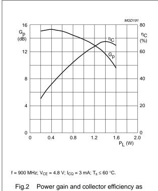
Fig.2 Power gain and collector efficiency as functions of load power; typical values.
