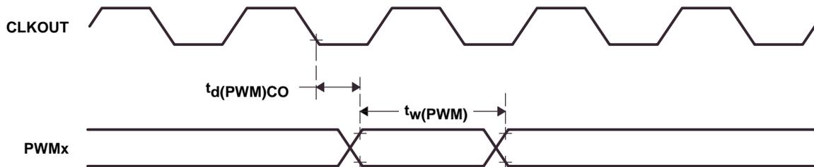
**Figure 34. PWM Output Timing**
