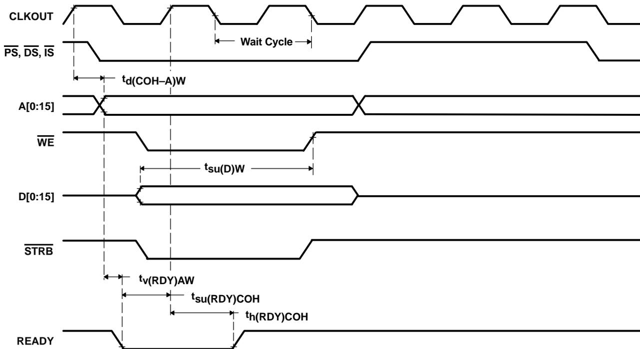
Figure 48. Ready-on-Write Timings
