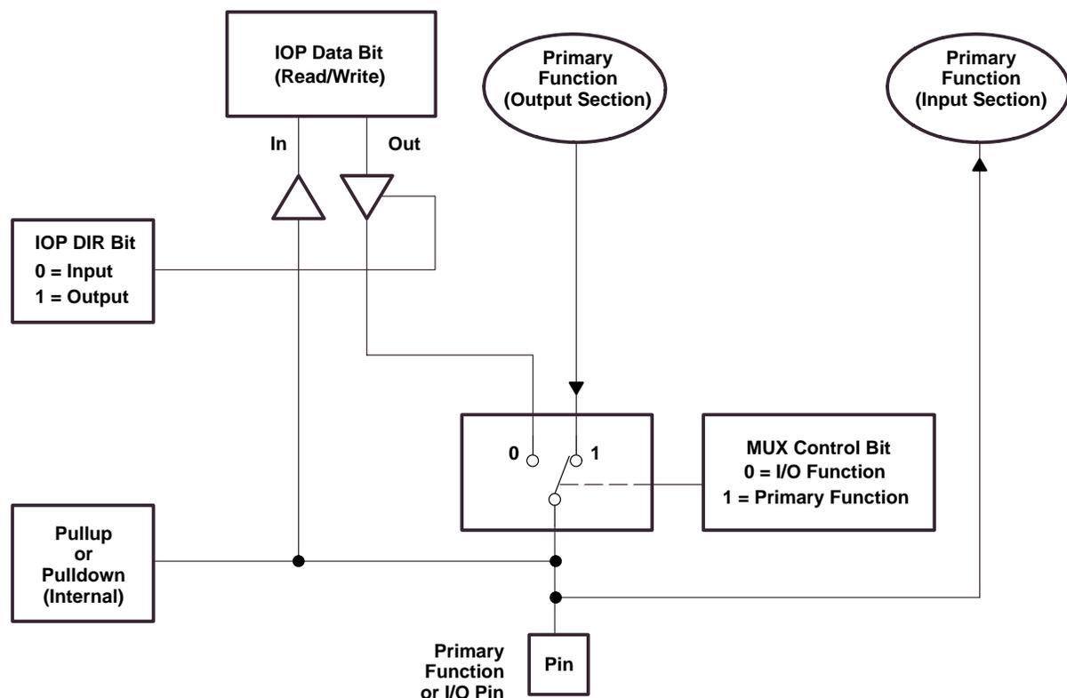
Figure 17. Shared Pin Configuration
