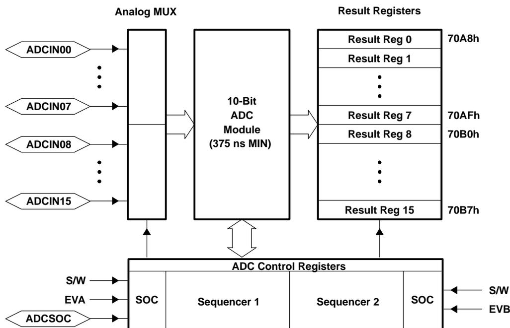
**Figure 11. Block Diagram of the 240xA ADC Module**
